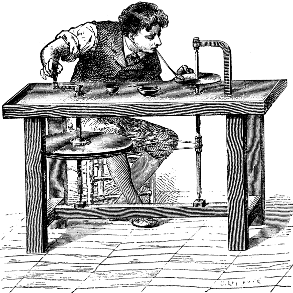
Fig. 125.—Apparatus for Sawing Hard Stones.
